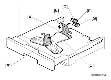
Four paper size switches [D] to [G], working in combination, detect the paper size as shown in the table below. The actuators are on the side plate [A]. The side plate is moved by the end plate [B] through a cam [C].
