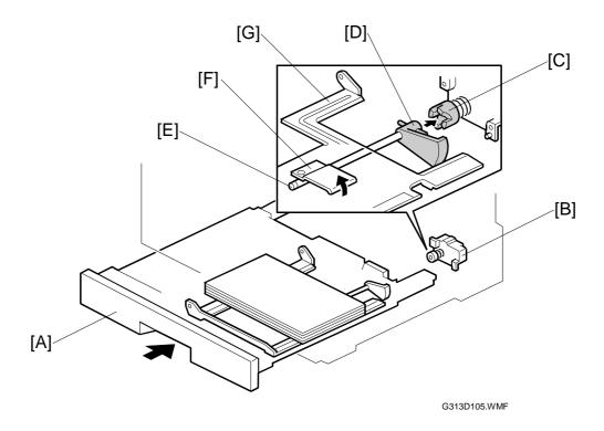
The paper size switches ( 2.4) detect when the paper tray [A] is placed in the machine. When the machine detects that a tray has been placed in the machine, the tray lift motor [B] rotates and the coupling gear [C] on the tray lift motor engages the pin [D] on the lift arm shaft [E]. Then the tray lift arm [F] lifts the tray bottom plate [G] until the paper lift sensor for the tray detects that the top of the stack is at the paper feed position.
